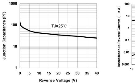
Fig.1-Typical Junction Capacitance
