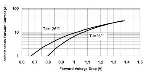
Fig.3-Typical Instantaneous Forward Voltage Characteristics
